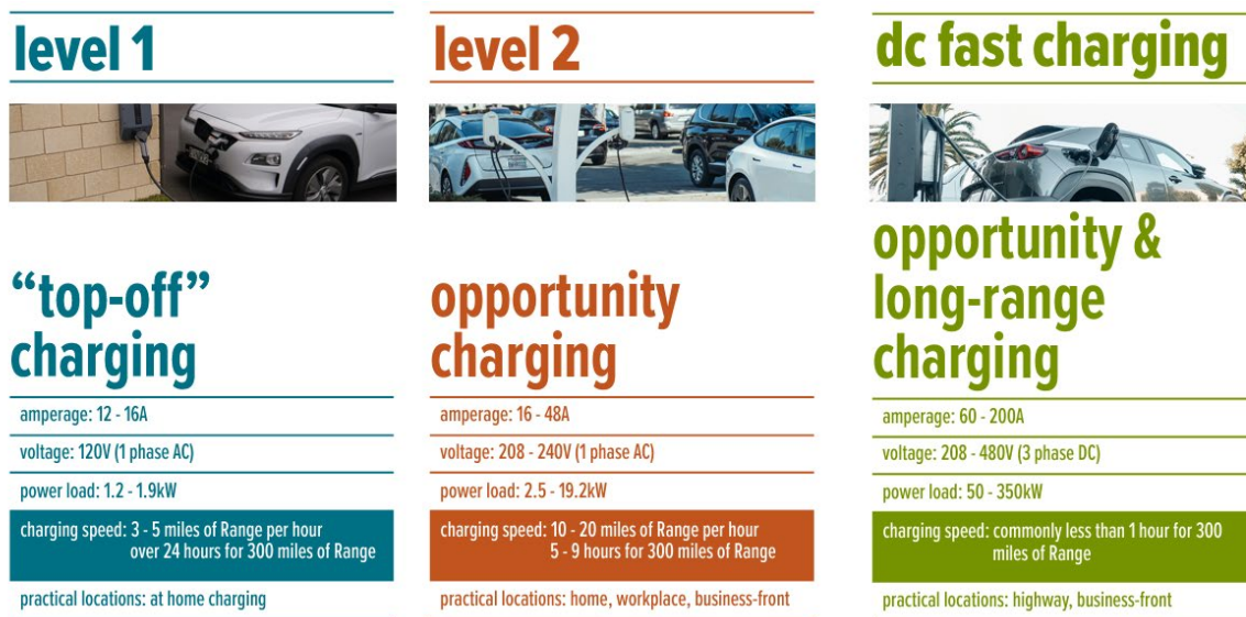
Figure #3.5. The three types of electric vehicle charging stations. Source: The Dynamic Sustainability Lab @ Syracuse University. lxxxviii
